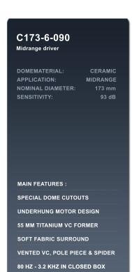
The C173 – 6 – 090 is a 6.5 inch midrange driver with ultra hard ceramic dome.
