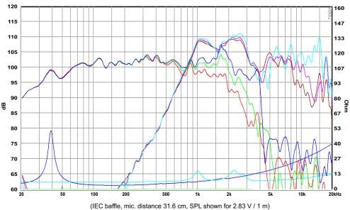
Response Curve: (Woofer) ----- (Blue): on axis ----- ( Green ): 30° off-axis ----- ( Red ): 60° off-axis (Tweeter) ----- (Blue): on axis ----- (Purple): 30° off-axis ------ (Brown): 60° off-axis
