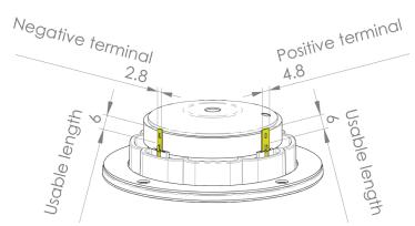
Terminal plating: Gold Thickness, both terminals: 0.5 mm
