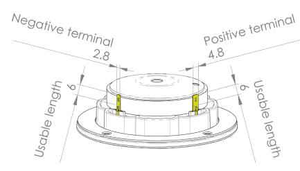
Terminal plating: Gold Thickness, both terminals: 0.5 mm
