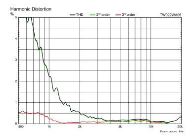
Measuring conditions, Harmonic Distortion Driver mounting: Infinite baffle Microphone distance: 0.5 m Input signal: Stepped sine wave, 2.83 VRMS Smoothing: 1/6 oct.
