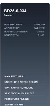
The BD25 - 6 - 034 is a 1 inch tweeter with ultra hard diamond dome in a 82 mm frontplate.
