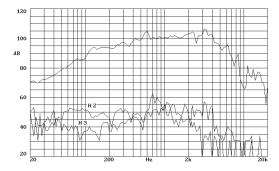
Note: on axis frequency response measured with loundspeaker standing on infinite baffle in anechoic chamber, 1w @ 1m.
