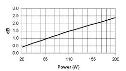
Note: These losses are calculated from a five minutes AES power test applying band limited pink noise (100-5000 Hz). The loudspeaker is free-air standing.
