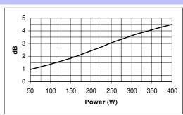
Note: These losses are calculated from a five minutes AES power test applying band limited pink noise (25-1200 Hz). The loudspeaker is free-air standing.
