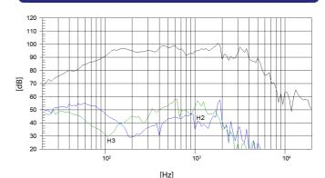
Note: On axis frequency response measured with loudspeaker standing on infinite baffle in anechoic chamber, 1W @ 1m
