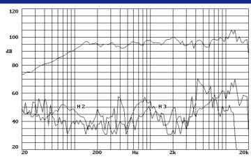
Note: On axis filtered frequency response measured with loudspeaker standing on infinite baffle in anechoic chamber, 1w @ 1m with FD2XA.
