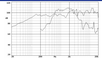
Note: on axis frequency response measured with loudspeaker standing on infinite baffle in anechoic chamber, 2.83V @ 1m.
