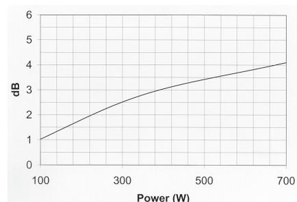
Note: These losses are calculated from a five minutes AES power test applying band limited pink noise (25-1200 Hz). The loudspeaker is free-air standing.
