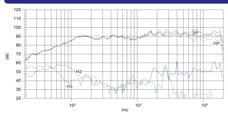
Note: Filtered frequency response measured with loudspeaker standing on infinite baffle in anechoic chamber, 1W @ 1m with FD-2CX
