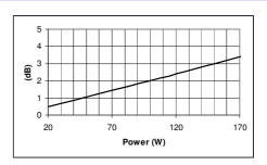
Note: These losses are calculated from a five minutes AES power test applying band limited pink noise (80-3500 Hz). The loudspeaker is free-air standing.
