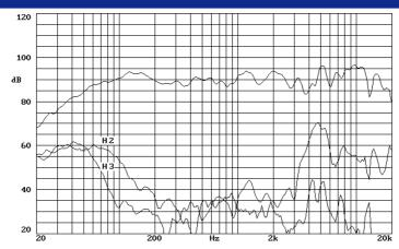
Note: on axis frequency response measured with loudspeaker standing on infinite baffle in anechoic chamber, 1w @ 1m. Crossover frequency set at 3,75 kHz @ 12dB/oct.
