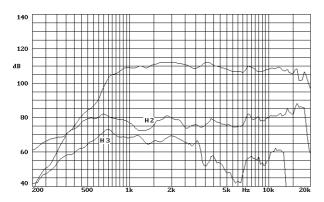
Note: on axis frequency response measured coupled to TD-164 horn in anechoic chamber, 2.83V @ 1m. Polígono Industrial Moncada II • C/. Pont Sec, 1c • 46113 MONCADA - Valencia (Spain)
