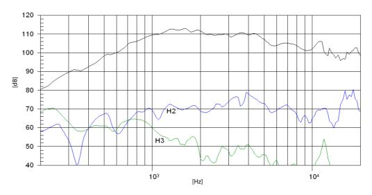
**Note:** On axis frequency response measured coupled to TD-385 horn in anechoic chamber, 2,83 v @ 1m
