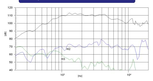
**Note:** On axis frequency response measured coupled to TD-365 horn in anechoic chamber, 2,83 v @ 1m
