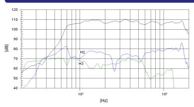
Note: On axis frequency response measured with CP-385/Nd standing on infinite baffle in anechoic chamber, 1W @ 1m
