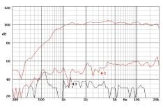
Note: on axis frequency response measured in an echoic chamber, 1w @ 1m.
