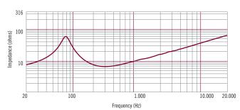
Impedance magnitude curve measured in free air.
