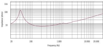
Impedance magnitude curve measured in free air.
