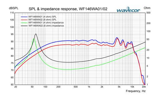
Measuring conditions, SPL Driver mounting: Flush in infinite baffle, back side open (no cabinet) Microphone distance: 1.0 m Input level: 2.83 V<sub>RMS</sub> Smoothing: 1/6 oct.
