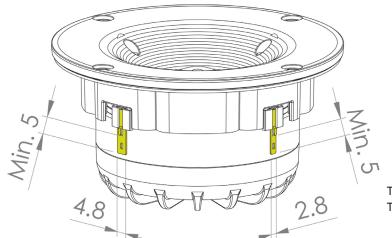
Thickness, both terminals: 0.5 mm Terminal plating: Gold
