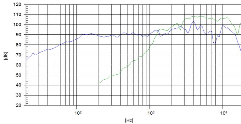
Note: On axis frequency response measured with loudspeaker standing on infinite baffle in anechoic chamber, 1W @ 1m
