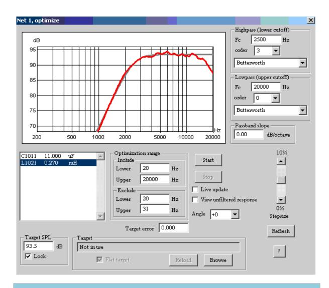
Example of 3<sup>rd</sup> order Butterworth filtering at 2500 Hz with two components.
