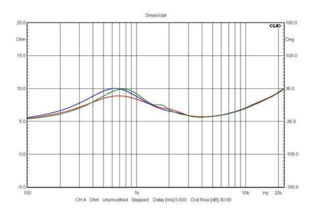
Impedance of 3 tweeters displaying low resonance frequency and modest rise in impedance due to magnetic oil in magnet gap.
