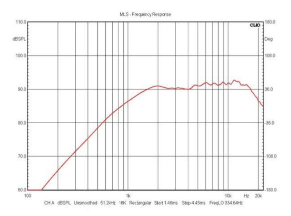
Frequency response from a more appropriate off-axis mounting on a 200 mm front panel with 7, 8 and 12 cm to nearest edges.
