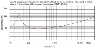
Impedance magnitude curve measured in free air.
