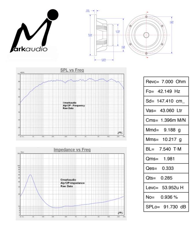
The recommended Max usable excursion = 5.4mm (non linear bass load) and Max power handling = 30 Watts (Nom).
