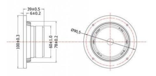
Installation: please note the off-set screw positions on the frame mounting.
