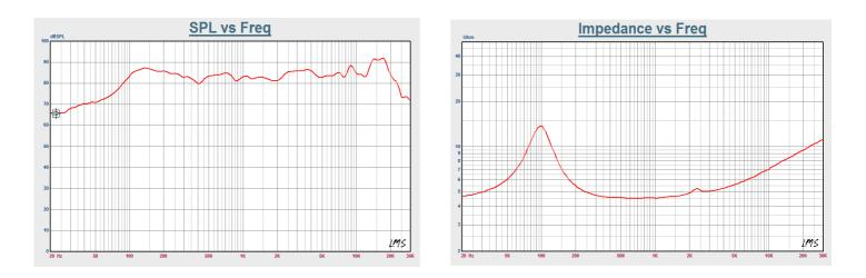
Revc= 3.600 Ohm Fo= 101.220 Hz Sd= 28.270 cm<sup>2</sup> Vas= 1.324 Ltr Cms= 1.166m M/N Mmd= 1.992m Kg Mms= 2.078 g BL= 2.522 TM Qms= 1.493 Qes= 0.755 Qts= 0.502 Levc= 38.886u H No= 0.181 % SPLo= 84.593 dB Xmax= 3.0mm 1 way
