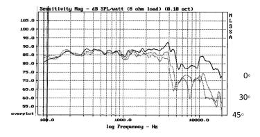
Measured on IEC baffle using Bruel & Kjaer 3144 model microphone.
