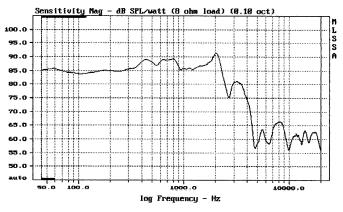
Measured on IEC baffle using Bruel & Kjaer 3144 model microphone.
