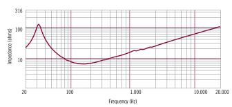
$\label{lem:lempedance} Impedance\ magnitude\ curve\ measured\ in\ free\ air.$
