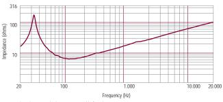
Impedance magnitude curve measured in free air.
