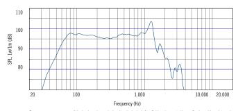
Frequency response curve of the loudspeaker make in a hemispherical, free field and mounted in a reflex box with an internal volume of 80 litres and tuned at 50Hz, applying a sinusoidal signal of 2.83 V @8 at 1m.
