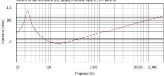
Impedance magnitude curve measured in free air.
