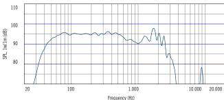
Frequency response curve of the loudspeaker make in a hemispherical, free field and mounted in a reflex box with an internal volume of 160 litres and tuned at 38Hz, applying a sinusoidal signal of 2.83 V @8 at 1m.
