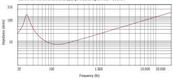
Impedance magnitude curve measured in free air.
