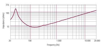
Impedance magnitude curve measured in free air.
