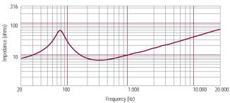
Impedance magnitude curve measured in free air.
