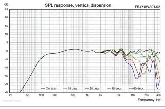
Download FR4X6WA01 on-axis SPL response as .txt file Download FR4X6WA02 on-axis SPL response as .txt file Measuring conditions, SPL Driver mounting: Flush in infinite baffle, back side open (no cabinet) Microphone distance: 1.0 m Hearth Sires 1, 2 92 We as a transed size wave
