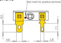
Thickness, both terminals: 0.5 mm Terminal plating: Gold
