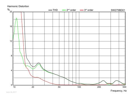
Measuring conditions, Harmonic Distortion Driver mounting: In sealed, heavily stuffed enclosure, internal volume 25 lit. Microphone distance: 0.5 m Input signal: Stepped sine wave, 11 VRMS (SW275BD01) / 15.5 VRMS (SW275BD02) Smoothing: 1/6 oct.
